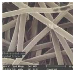
Synthetic Coarse Fiber (400X Magnification)
